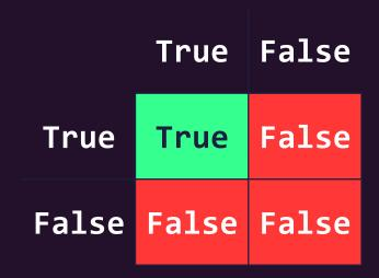
You read a truth table like a multiplication table. Start with a finger on one column label and one row label, per each side of the operator, and trace your way in.
